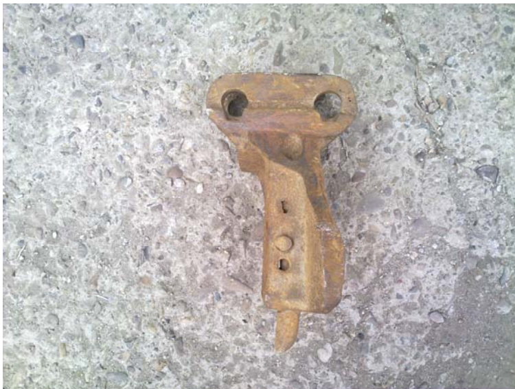
Figure 7: Scraper at the maximum wear limit in mounted on scraper shovel state.
