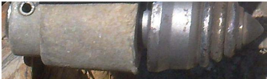
Figure 13: Scraper bolt, mobile (rotating) and interchangeable (see Fig.12, Item 3)
