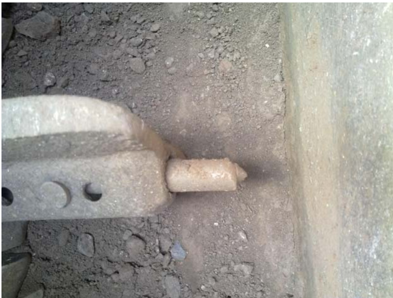
Figure 9: Wear forms of the active part of fixed scrapers with sintered metallic carbide.
