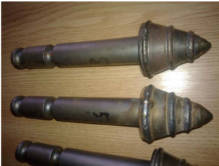
Figure 11: Scraper type MCB-450 loaded with extremely tough alloy powders through laser melting
