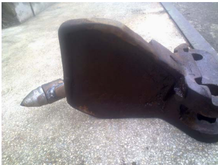
Figure 14 (a): A new chain section with the new type of scraper with sintered metallic carbide – the front side
