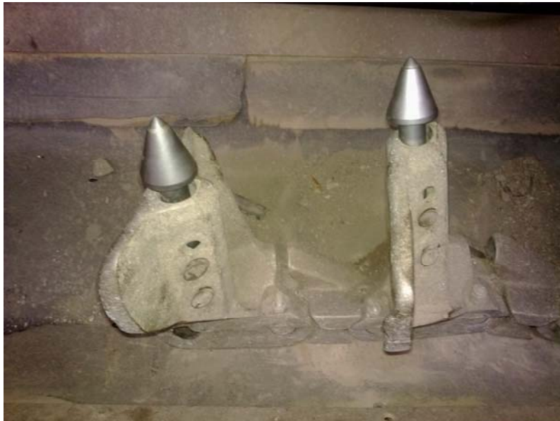
Figure 10: Improved version of the scraper for the excavation chain type MCB-450.
